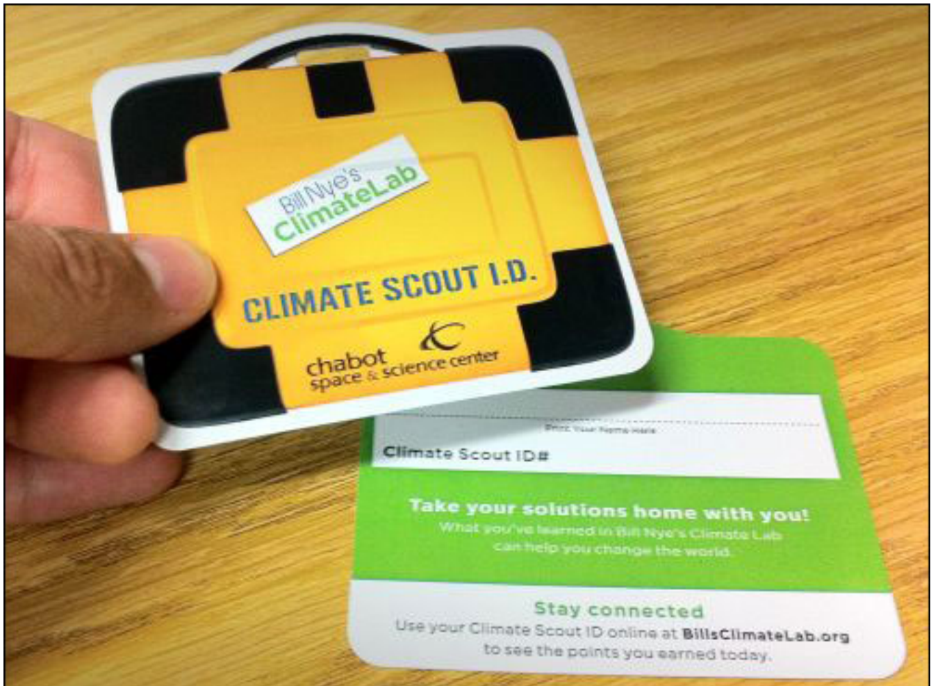
Each Climate Scout ID card has an embedded Alien Technology EPC Gen 2 inlay. (Photo courtesy of Proximity Lab)
